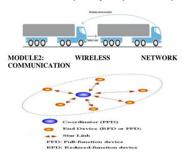
Wireless pan(WPAN) focuses on low-cost, low-speed ubiquitous communication between devices. WPAN has a range of 10-100 meter communications area which Transfers at a rate up to 250 Kbit/s.It is also used for secure communications and can be used in any topology that Uses Offset Quadrature Phase Shift Keying (OQPSK) modulation. WPAN uses 2400-2483.5Mhz frequency band
